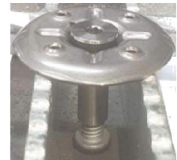
Correctly Installed and Tensioned T-Clip
